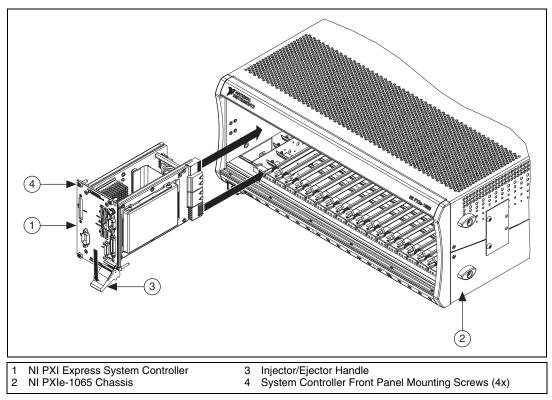
system controller to the rear of the chassis, making sure that the injector/ejector handle is pushed down as shown in Figure 2-3.
